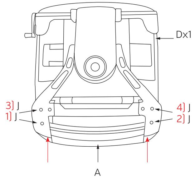
Align Back Frame mounting holes on both sides
